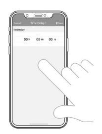
Time Delay 1 is the amount of time the Motion Event lighting level remains ON while the sensor does not detect motion. If the sensor does detect motion, Time Delay 1 is reset and begins counting down again.
