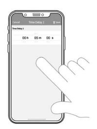
Time Delay 2 is the amount of time the Standby lighting level remains ON while the sensor does not detect motion. If the sensor does detect motion, the Motion Event dimming level is activated and Time Delay 1 begins counting down again.
