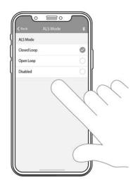
Ambient Light Sensing is the ability of the sensor to detect ambient light, and appropriately dim associated lights to maintain constant comfortable light levels.
