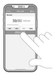
The Standby Level is the dimming level a light will go to after Time Delay 1 has expired when the Standard MS Mode is selected.
